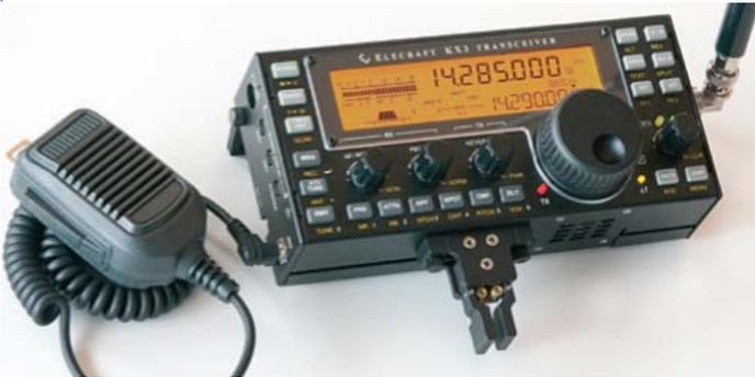
Advanced DSP Dual Watch / Noise Reduction / Noise Blanking / Autonotch / Stereo Audio Effects / PSK31 / RTTY with or without a PC
