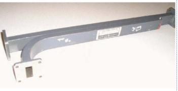
Pict. 2 — HP X785D Waveguide Directional Coupler
