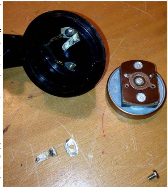
Fig. 14 Broken contact piece inside American phone
