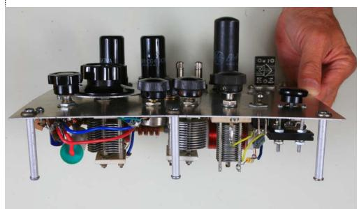
I followed the original schematic as reproduced here. adopted except that VE7SL's excellent suggestion regarding isolating the B+ voltage from the variable capacitor for the transmitter section as you see below. The original schematic calls for connecting the B+ voltage to both the rotor and stator sides of the capacitor which runs the risk of inadvertent electric shock.
